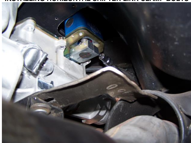
INSTALLING HORIZONTAL SHIFTER LINK CLAMP BOLTS
